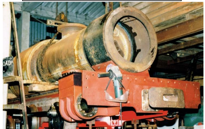
trial boiler assembly to frames
